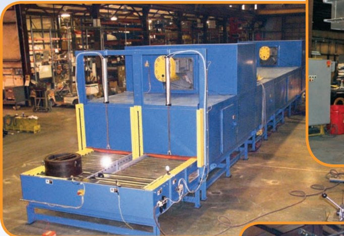
Custom conveyor oven featuring pop-up 90° transfers and zero pressure product accumulation inside the oven
